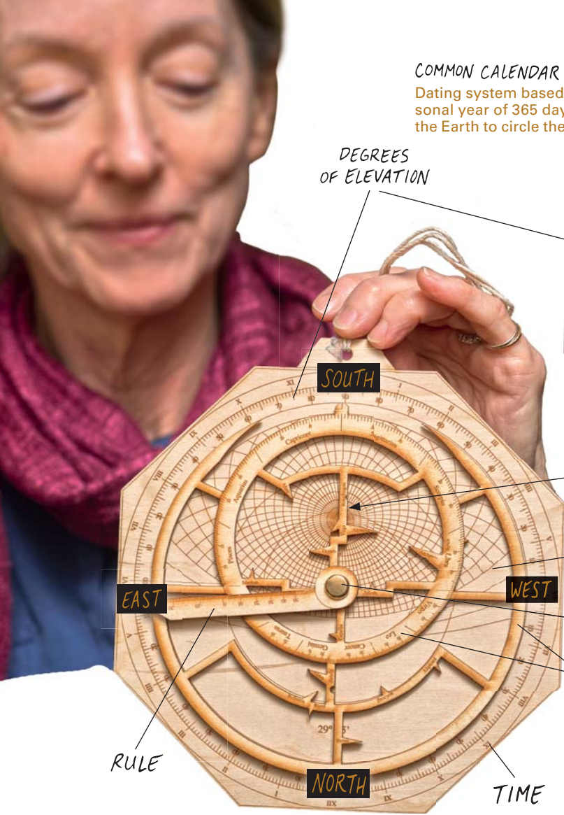
The author holds her astrolabe, laser fabricated from wood with a zenith calibrated to the latitude of Houston, Texas, above; its back side appears above right. In 694 AH (1294–95 CE), Mahmud ibn Shawka al-Baghdadi produced this astrolabe, opposite.
