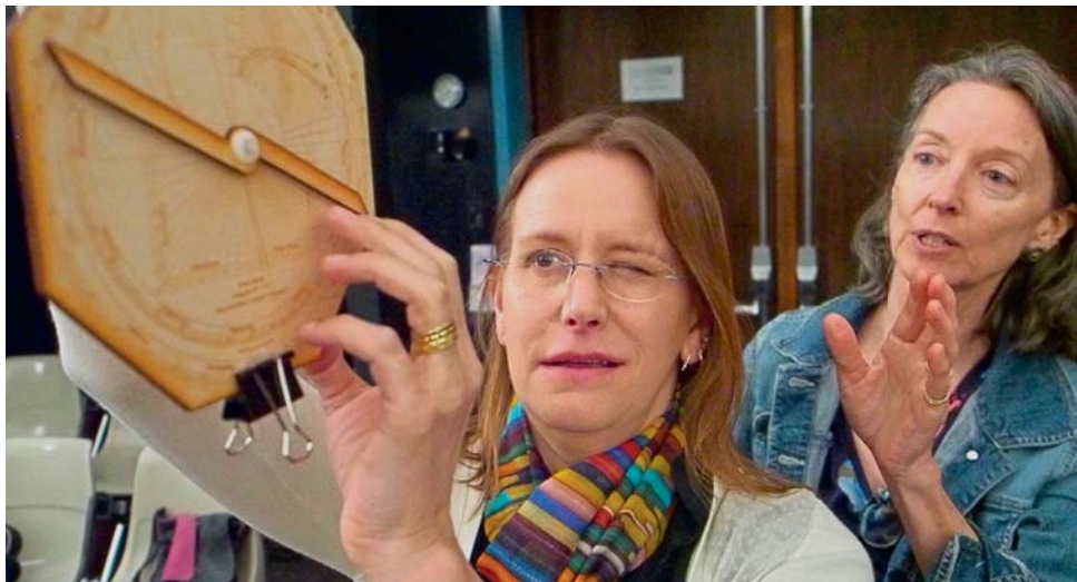
The author guides her stepdaughter, Isa, as she sights along the astrolabe's alidade to calculate the height of a balcony in an auditorium at Central Connecticut State University.
