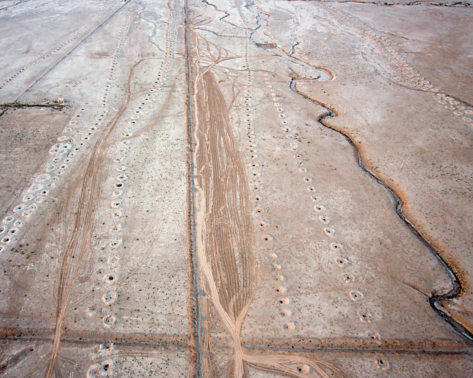
In Turpan, which lies below sea level, numerous qanats, such as these above, convey water from the foothills of the Tien Shan Mountains to cash crops such as grapes, which are dried into raisins in buildings such as these, left.
